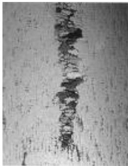
A freckle defect in solidified metal
