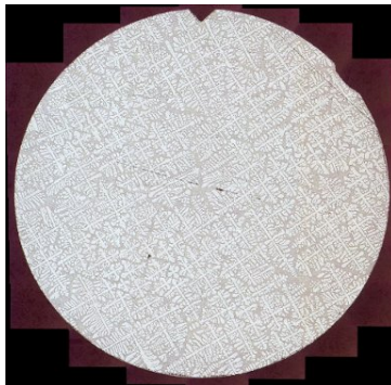
Dendrite microstructure from terrestrial experiment, courtesy of Surendra Tewari of CSU
